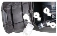
4. Carefully cut the end of the **GARDEN HOSE** to expose the hose barb (4) and internal spring (5). The **GARDEN HOSE** can now be removed from the reel and a new hose inserted through the layering mechanism of the reel.
