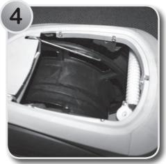
Ensure that both locking bars (on each side) are placed securely in the holes on the auto wheel before proceeding.
