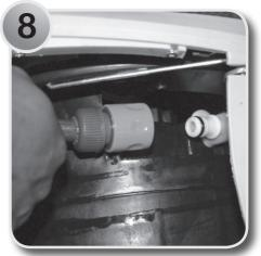
Detach the hose connector from the 'quick release' snap on connection.
