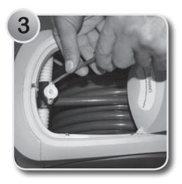
Taking a cross head screw driver, unscrew the 2 screws holding the guide hole in place slighly, so the hose moves freely as you extend it.
